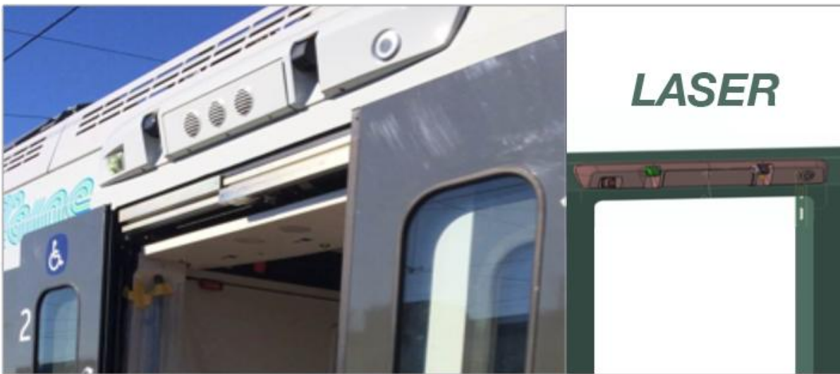
■ Lasers mounted next to the door
