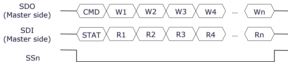
Figure 2 : SPI frame structure
