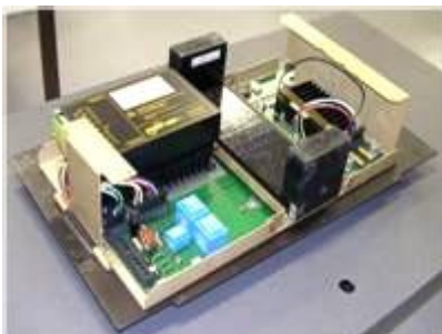
KFSI track antenna (inside view)
