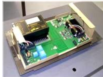
KFSI track antenna (inside view)
