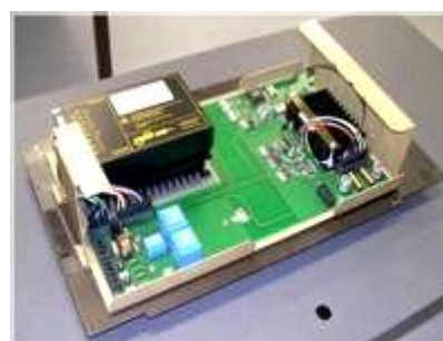
KFSI track antenna (inside view)
