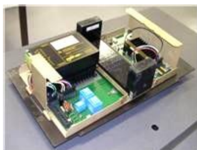
KFSI track antenna (inside view)
