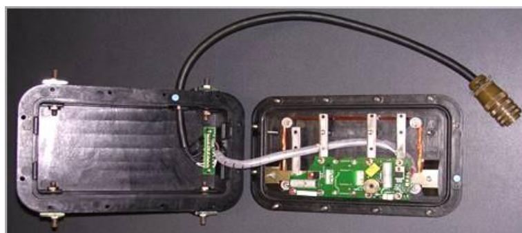
Internal view of an KFS Sensor
